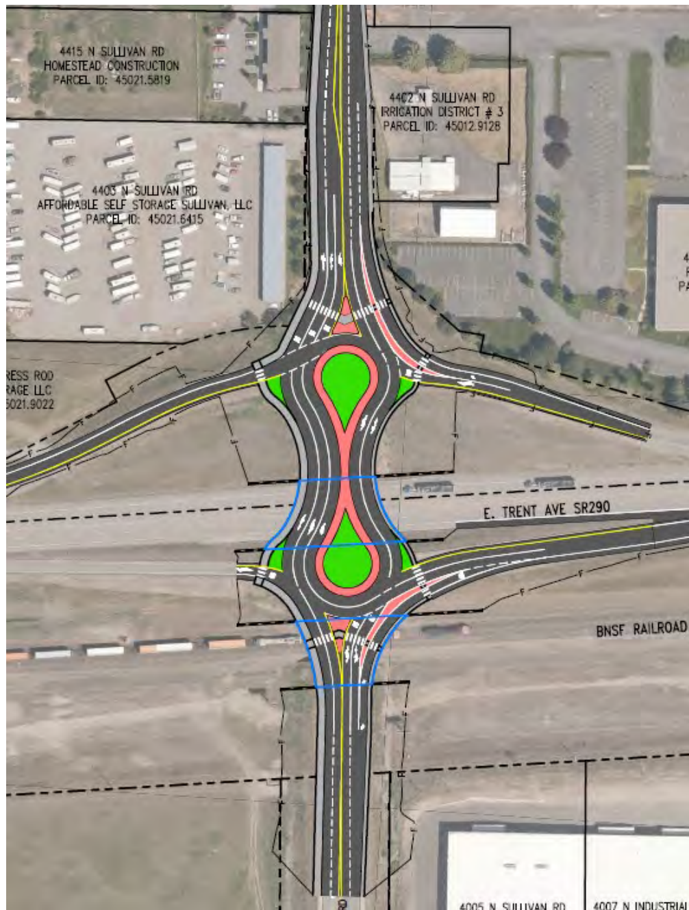
Figure 4. Alternative 2: Diamond Interchange with Peanut Roundabout
